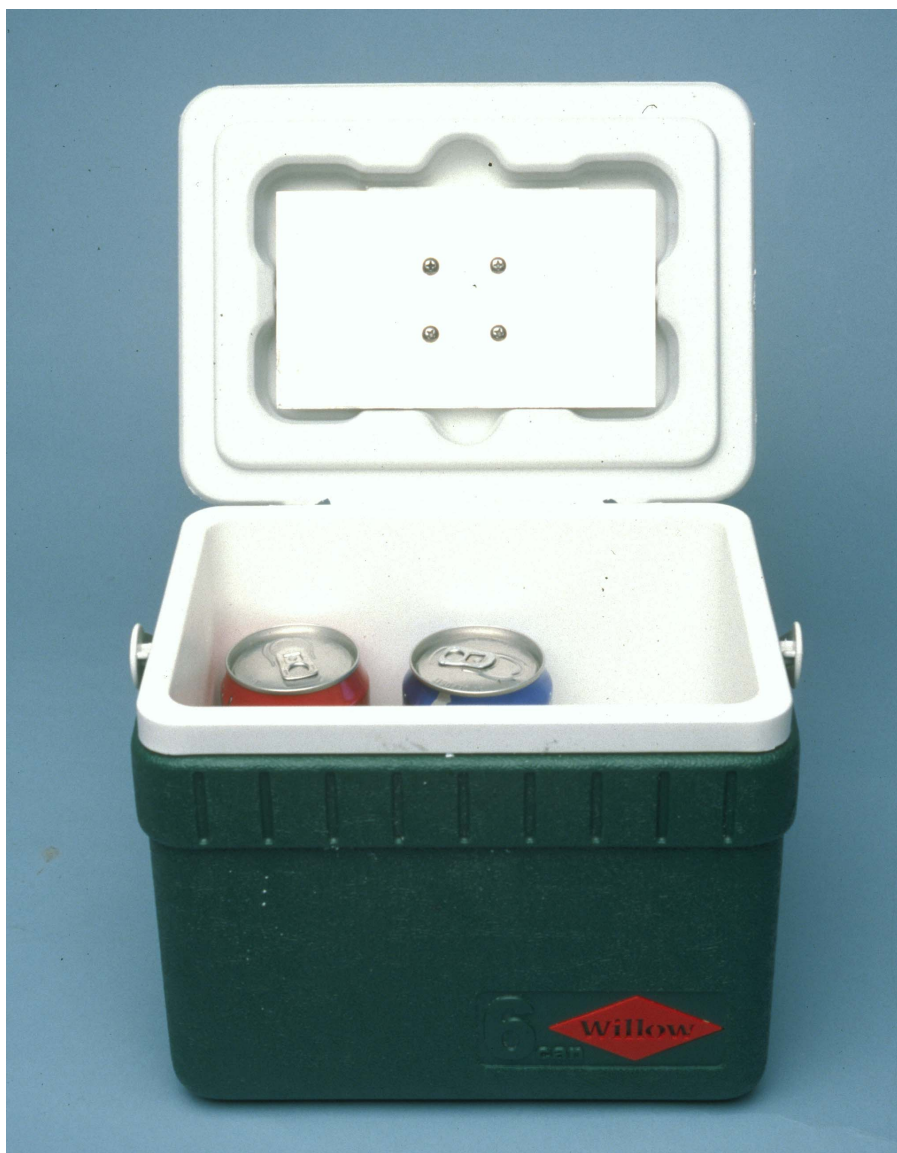
(Above): the Peltier module attached to the top of the cooler lid while below is the view from inside the cooler.
