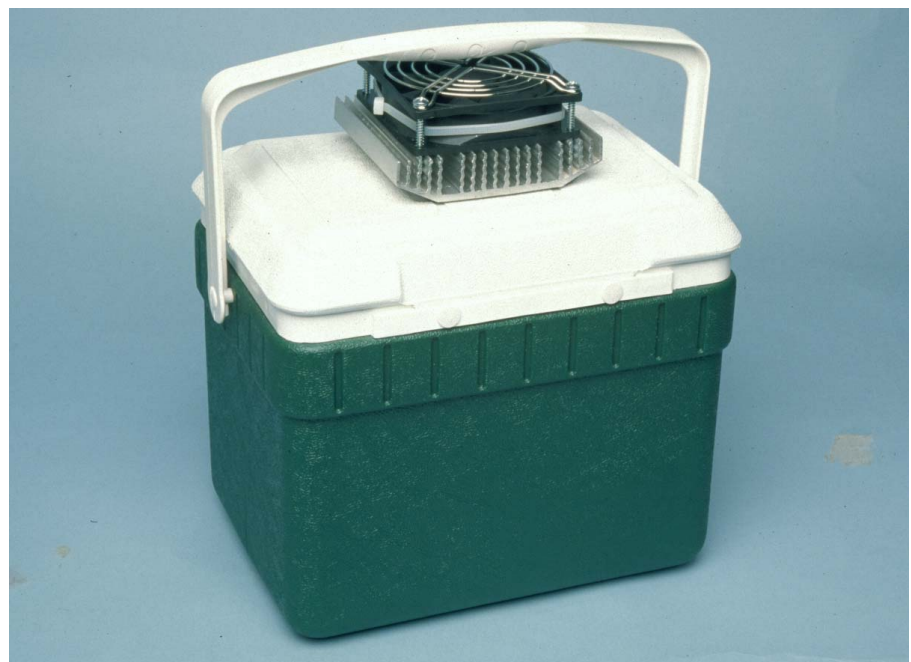
Just in case you haven't seen one before, this is what the Peltier device looks like. This is a lower rated device than the one in this module.
